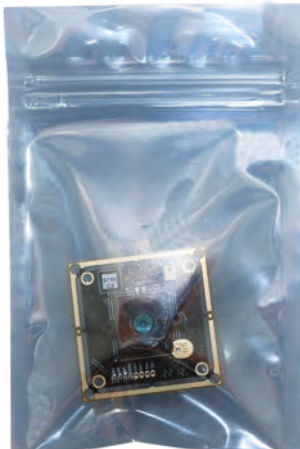
Place Camera Sample into Anti-Static Bag
